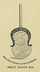
Of course, a special shape of tyre is used with these, and their object is to prevent all possibility of the tyre coming out, and at the same time to give greater downward depth of rubber. They would be the best thing out for the steering wheels of tricycles, but they are made too thin in the centre, and are not yet perfected in manufacture, consequently they "buckle" easily. When right, they will undoubtedly be the best form of rim extant for all wheels subject to severe side pressure.
